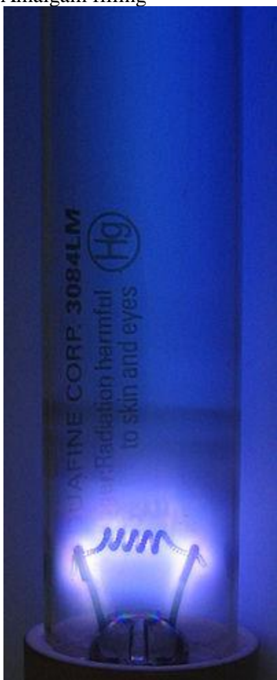
☐ The deep violet glow of a mercury vapor discharge in a germicidal lamp , whose spectrum is rich in invisible ultraviolet radiation. See also: Amalgam (dentistry)
